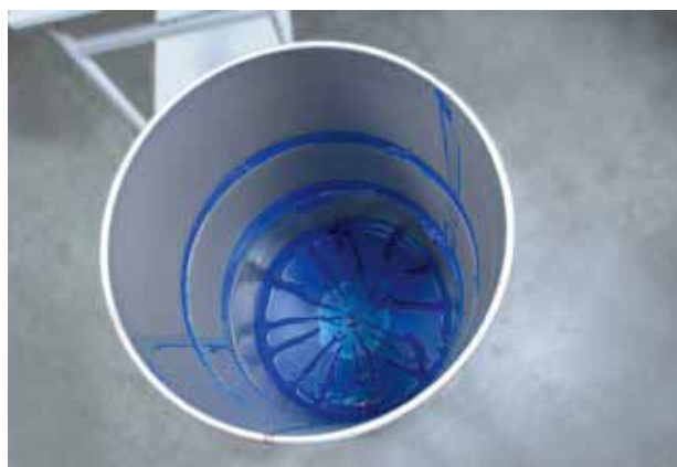
Emptying of drums to less than 1 % residue.*
